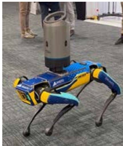
Robot – used to find radioactive material.
